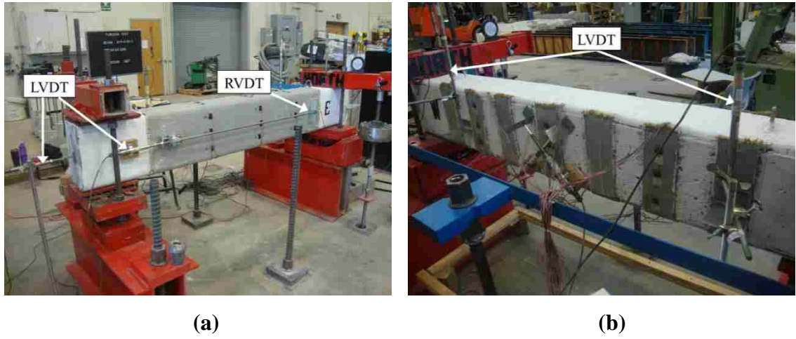
Figure 6. External instrumentation on a) east side, b) west side of the beam.
